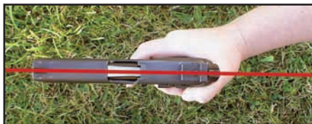
When the gun is large for the shooter's hand, recoil will go into (or beyond) the thumb's basal joint and the gun will not align with the arm bones.
