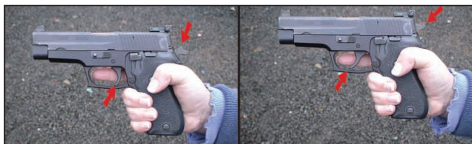
DA/SA trigger reach should be measured in DA mode, since the gun will most likely be in DA mode if needed for defense.
