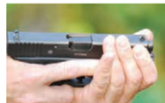
Once out of battery, a Glock will not fire.
