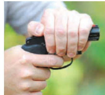
Grabbing the cylinder can keep the revolver from firing.
